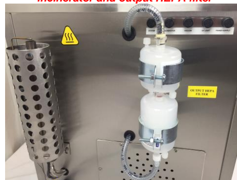
incinerator and output HEPA filter
