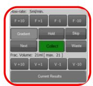
During the separation *Run* (or *Extended Run*) some buttons will be disabled or hidden. Some more complex operations are allowed only in *Pause* (or *Extended Pause*) state (e.g. Gradient, Detection...).
